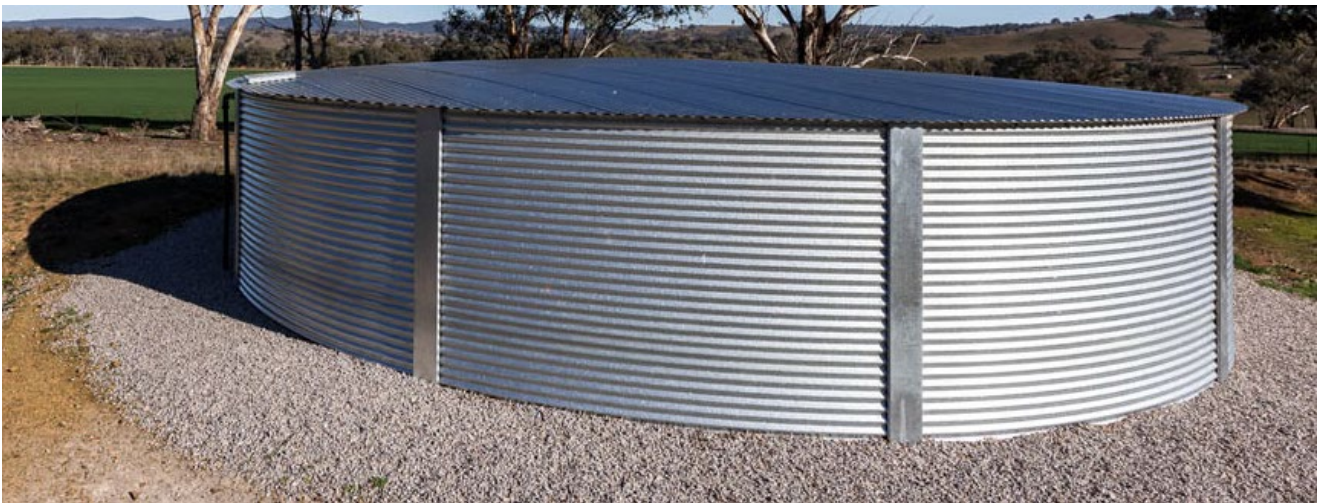
Figure 1 Aggregate should be at least 800mm from the base of the ClearWater Tank and 75mm deep.
